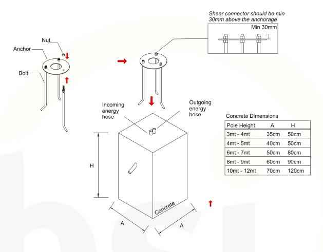
4) After the concrete has been dried, the electrical cables are pulled and the nuts are removed.
