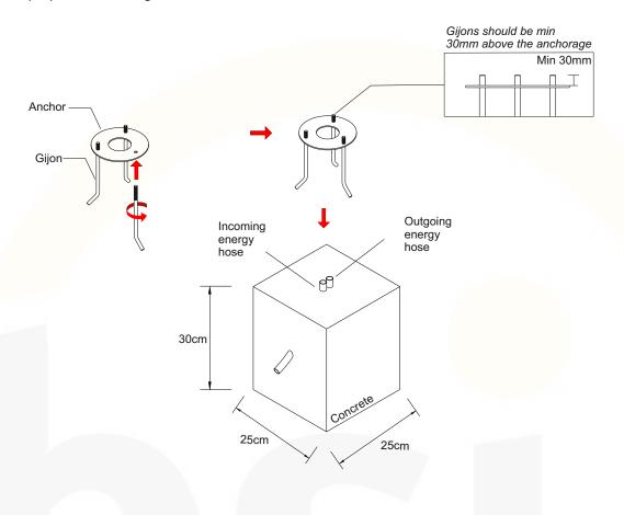
2) After the concrete has been dried, the electrical cables are pulled.
