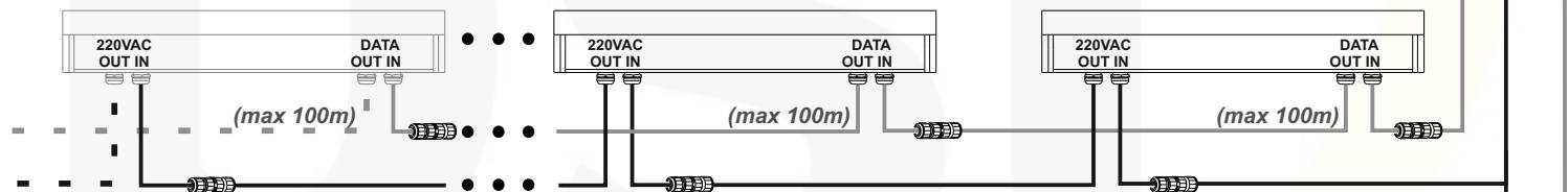
\*The luminaires make automatic addressing. It doesn't need any sorting.
