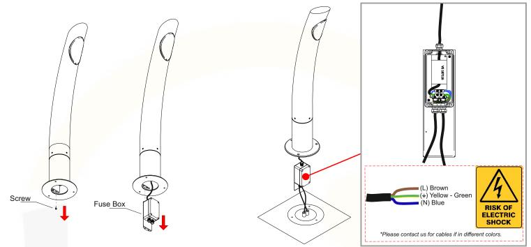
4) -The fuse base is screwed back into place.
