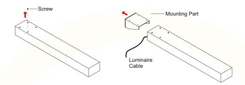
4) The mounting part is screwed onto the pole.
