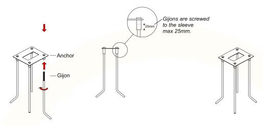
2) - The prepared anchor is embedded in the concrete and leveled. - After the concrete is dried, the energy cabling is done.
