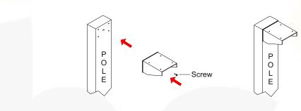
5) -The cable is passed through the cable hole and passed into the pole. -The luminaire is fastened to the mounting part and the screwed from the top.
