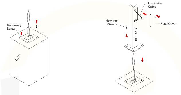
7) Electrical connection is done and the fuse cover is screwed
