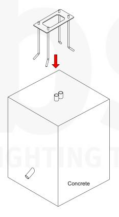
4) After the concrete is dried, the energy cable is done.
